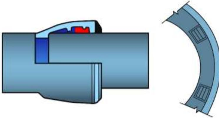
The tyton-sit anchor must only be used with a tyton socket profile joint and cannot be used with a Rapid or AJ type socket profile.
